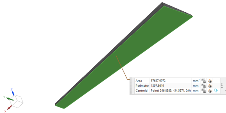
Figure 31: Wing area calculation in NX, used to back out the cruise pressure.
