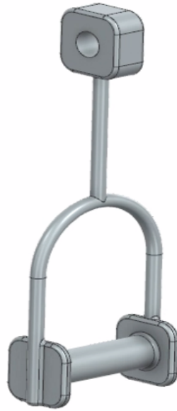
Figure 12: Rear landing gear linkage.
