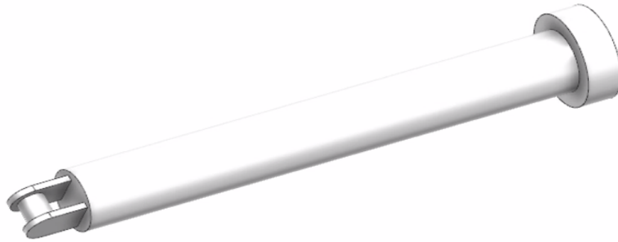
Figure 14: Hydraulic actuator outer cylinder with pin connection.
